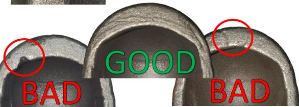
Critical area to be 100% inspected -Any crack Rejected
