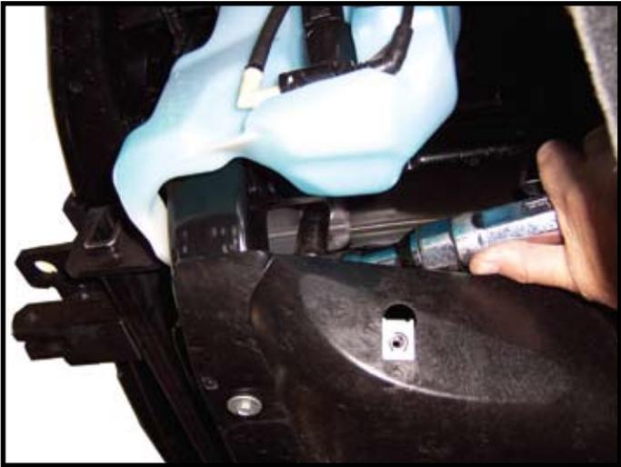
**20.** With an assistant, install baseplate up against bottom of frame. (Make sure sensor wire is in front on cross-member.) Fasten using four 10mm flat fender washers, 10mm lock washers and 10mm-1.50 x 35mm bolts, thread into existing threaded holes in frame, **NOTE:** Use blue **LOCTITE**® on all bolts and tighten all bolts according to chart on front page.
