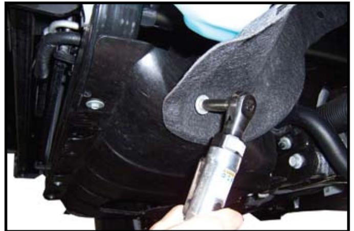
8. On drivers side, remove one bolt from front of wheel well to the side of skid plate to gain access to rear baseplate mounting hole. Repeat for other side if equipped with tow hooks.
