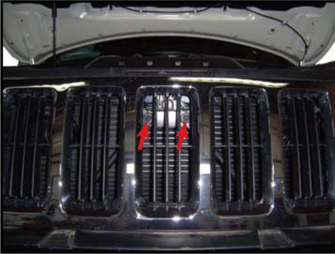
15. Remove two bolts from top bumper supports from behind grill. **NOTE: Be careful not to damage radiator.**
