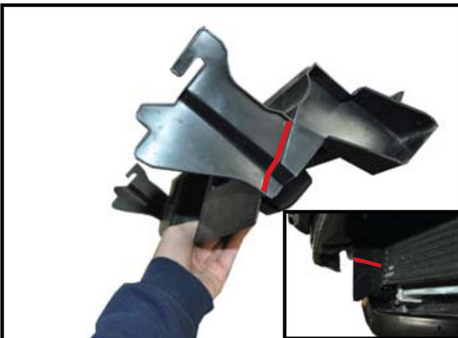
8a. **2014 and later:** trim air deflector as shown by cutting on each side on line as shown in picture and on passenger side cut air deflector attached to radiator as shown by line in insert picture.
