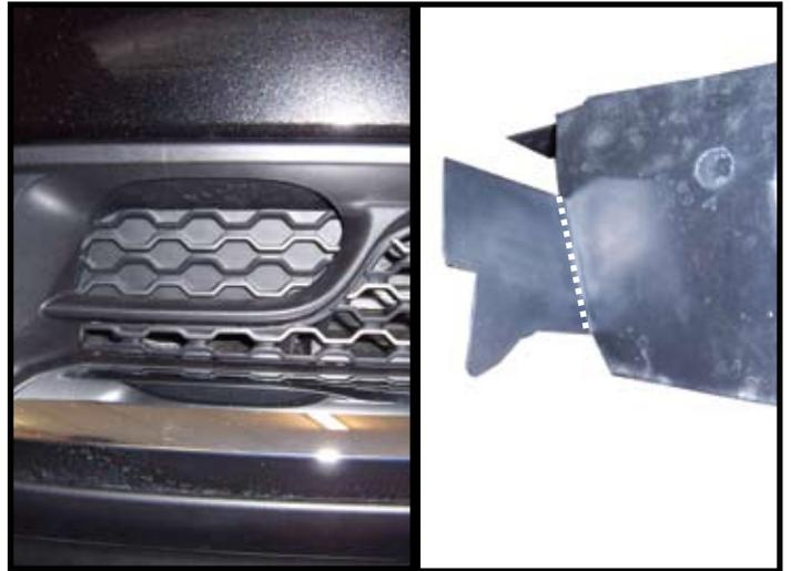
7. Remove tow hook covers if equipped, and cut the air deflector as pictured with dotted line.
