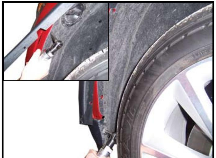
3. Remove one screw from fascia by trim molding and one screw from inner wheel well to bottom of fascia.
