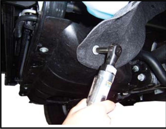
9. On drivers side, remove one bolt from front of wheel well to the side of skid plate to gain access to rear baseplate mounting hole. Repeat for other side if equipped with tow hooks.
