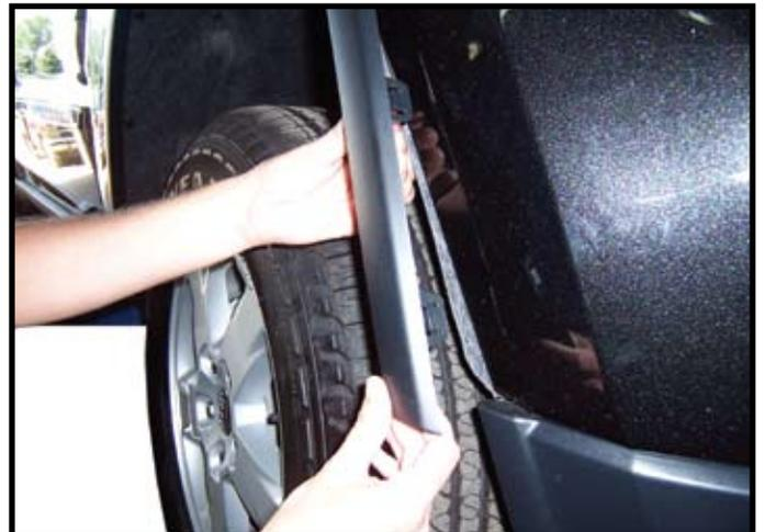
2. Carefully pull out on molding trim attached to side of fascia.
