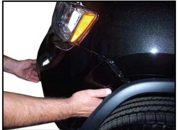
5. Carefully pull fascia out on each side by fender and pull fascia forward to remove. Unplug fog light if equipped.
