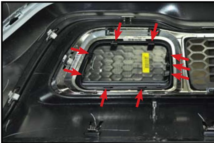
**20a.2014 and later:** Release tabs on back side of facia as shown by arrows to remove inserts to allow pullears to pass through facia if not equipped with tow hooks.
