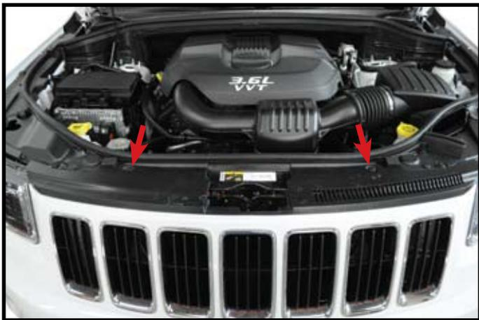
3. **2014 and later:** remove three plastic push fasteners from top of grill and release top of grill.
