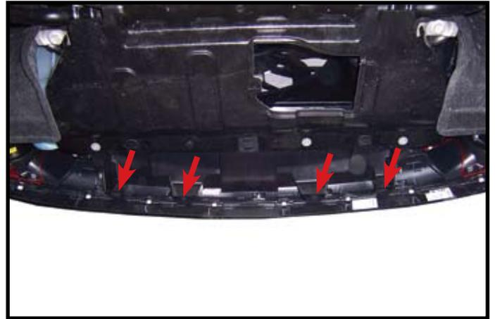
4. Remove four plastic push fasteners from bottom of fascia.
