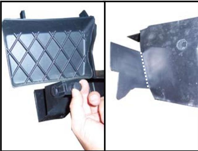
8. Remove tow hook covers if equipped, and cut the air deflector as pictured with dotted line.
