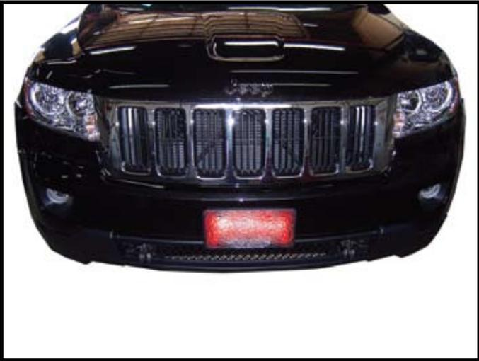
21. Reinstall adaptive cruise control sensor (if equipped), air deflector, fascia and plug in fog lights. Use the plastic rivet instructions to install the supplied rivets to fascia.
