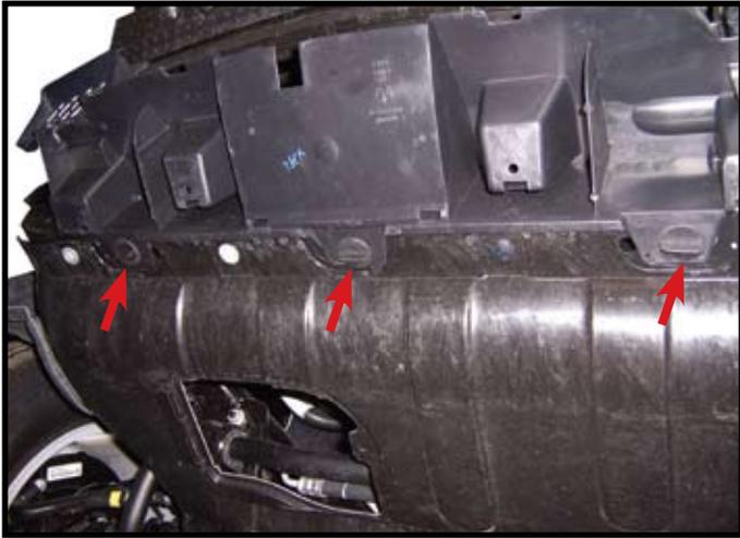
7. Temporarily remove air deflector by removing three turn clips. **NOTE:** Some years use plastic push fasteners.
