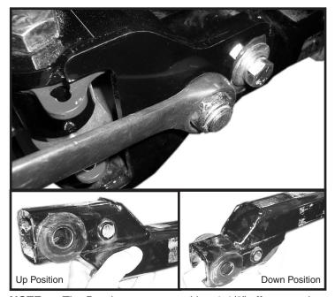
**NOTE:** The Dominator comes with a 1-1/2" off-set receiver that can be flipped to help level the tow bar with the towed vehicle. The receiver is in the down position from factory, to change to the lower position, remove both 1/2" bolts and washer from side of receiver joint head. Remove the 3/4" nut and bolt, slide receiver out of receiver joint head and flip receiver into the down position. Slide receiver back into the receiver joint head and reinstall the fasteners.
