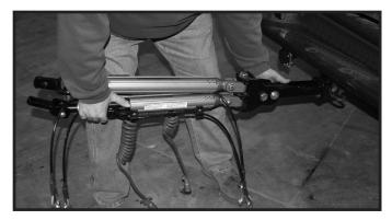
**Step 2.** Insert the Dominator into a Class III or IV hitch. CAUTION: Tow bar must be inserted directly into tow vehicle receiver or into an approved rise drop receiver only! Tow bar should never be inserted into a receiver extension, bike rack, storage rack, motorcycle rack, or any other device that extends the tow bar away from the tow vehicle.
