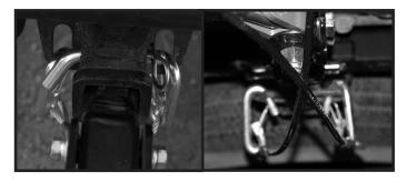
**Step 3.** Insert receiver pin through receiver until pin passes through. Secure pin with the Receiver hair pin. Crisscross safety cables underneath pivot assembly and attach to chain anchors on towing vehicle. Do not use coiled safety cables with this tow bar, always use straight Demco safety cables.
