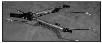
**Step 1.** Out of the box, the Dominator tow bar is setup for the recommended positions for the safety cables and light wire storage rod. These can be positioned to new areas to fit your setup by loosening the screw on the retaining rings and sliding them off the rail and relocating to a new position and tighten screw. Install the light cable (optional) by placing the coil over the wire support rod. Secure the cable with the cable locking hair pin.
