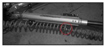
**Step 7.** Leave the electrical cable storage pin (circled above) out for the locking procedure in step 6. When step 6 is completed, position cable on storage rod leaving enough slack, and insert pin.
