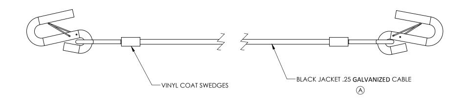
UNLESS OTHERWISE SPECIFIEDALL DIMENSIONS ARE IN INCHES DRAWN BY DATE THE DRAWING AND ALL INFORMATION THERE ON ARE THE PROPERTY OF DESCRIPTION JK 10/31/08 JCN 03/18/19 DRAWING. NO. 13273 SAFETY CABLE 54" 7000# RATING THIRD ANGLE DE FROJECTION TOLERANCES  $.X = \pm .060$   $.XXX = \pm .010$  NON-MACHINED  $.XX = \pm .030$   $.XXX = \pm .005$  MACHINED VOLUME 11.36 SCALE SHEET MIN. MACHINE SURFACE 250
