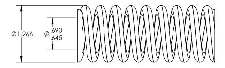
TOTAL COILS = 10.50 ACTIVE COILS = 8.50 FREE LENGTH = 3.500 SOLID HEIGHT = 1.90 CLOSED & GROUND ENDS 740 #/INCH DEFLECTION
