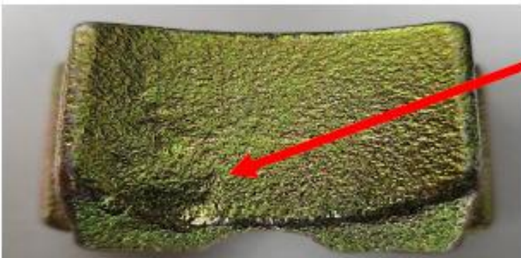
Example of nonconforming ball clamp
