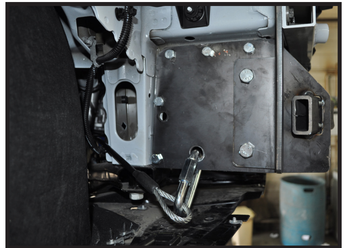
13. Drill three 3/8 holes on each side of the baseplate. Install 3/8 x 1" bolts and tighten.
