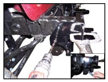
4. Using baseplate as template, drill 1/2" hole thru side of baseplate on each side. Install 1/2" x 1-1/2" bolt, 1/2" flat washer, 1/2" lock washer, and nut strip. Nut strip goes on frame side and bolt and washers thru baseplate side. Tighten bolts according to torque chart on front page. Note: Use LOCTITE® on all bolts and nuts.
