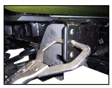
3. Put baseplate up from passenger side pushing tight towards driver's side. Align front slotted holes in baseplate with round holes of vehicle's bumper flange. Clamp each side so baseplate doesn't move. NOTE: Baseplate mounts on the outside of the passengers frame and the inside of the drivers frame.
