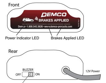
Buzzer ON/OFF (7 second delay)
