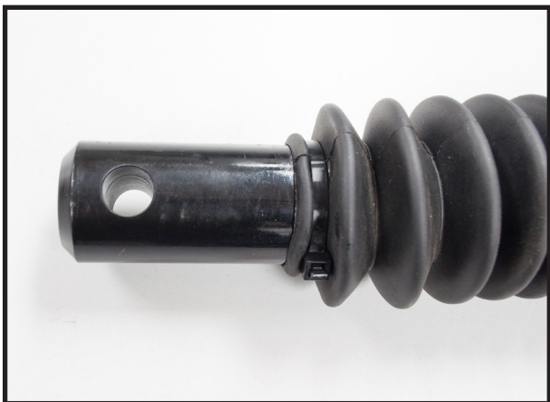
5. With the hole facing up with tow bar, place the rubber boot over adapter and use the supplied plastic tie to clamp boot to adapter. Cut unused plastic tie.
