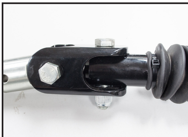
6. Bolt tabless clevis to adapter making sure not to over tighten, the clevis should rotate freely.
