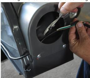
Pull all wire from light hole in housing and install the snapper hose clip approximately 1-1/2" back from end of wire shielding. Squeeze snapper clip tight with pliers.
