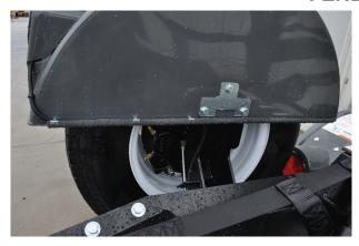
Install fender backup plate and three 3/8 x 1-1/2" bolts. Put nylon lock nuts inside of fender and tighten.
