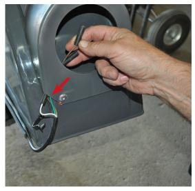
3. Router wiring in through back of tail light housing on the bottom inside of housing. Fish the three wire inside of housing.
