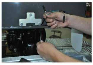
2. Fish the three wires from the mainframe through the rear hole in the fender trough.
