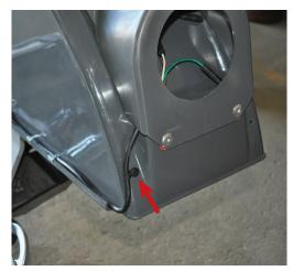
5. Push wires back into housing and finish routing wires in wire trough of fender and attach cable hanger. Install two metal wire clips using pliers. Place one clip 5-1/2" from rear of fender and one 8" from rear of fender (see red arrow).
