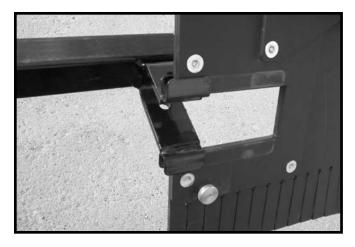
**3.** Slide the left & right rock guard onto the mounting slide channels. Note: If the center section is not bolted together, use three T-nuts and .25 x .50 phillips head screws to fasten center section together. (See parts breakdown) (Apply thread lock to threads)
