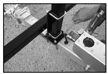
**1.** Attach upright postto tow dolly tongue, approximately 40" from tongue channel on tow dolly's main frame. Attach using two 3/8" x 3" x 4" u-bolts and four 3/8" nylon lock nuts.
