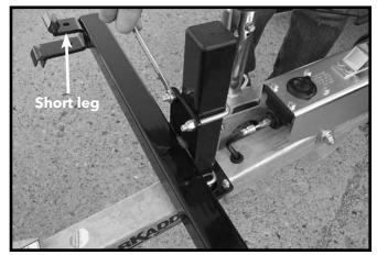
Install crossmember to upright post, making sure the short leg of the mounting channel on tube ends, is on top
