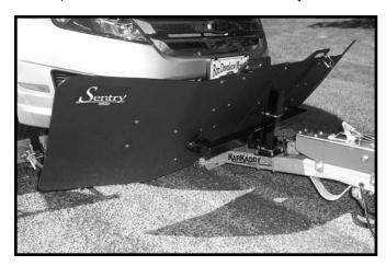
**6.** Once adjusted, the Sentry brackets can stay on tow dolly and the Sentry can be removed and placed in it's bag when not in use.
