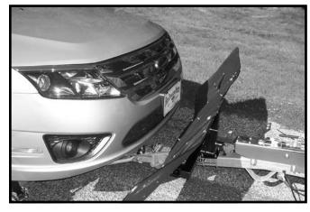
**5.** Adjust the mounting brackets on the tongue so the Sentry deflector is about 6" from the vehicle and the bottom of Sentry is about 1/4"-1/2" from the tongue of tow dolly.
