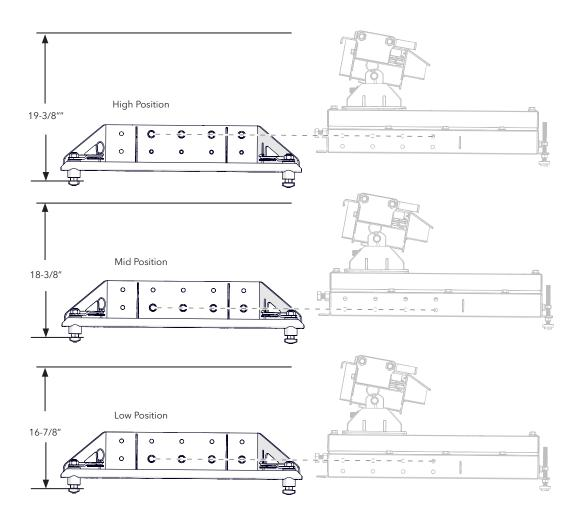
**IMPORTANT NOTE:** Incorrect mounting of the side plates to the main body will result in the incorrect position of the hitch for towing and will not allow the hitch to travel back to its full ability.
