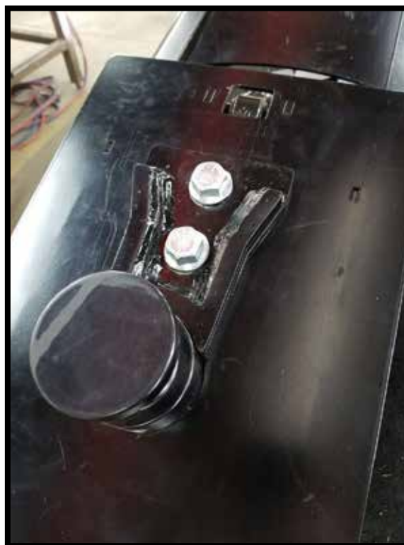
4. Place the 5/8" Grade 5 bolts and 5/8" nuts onto the locking plate as shown. Torque the bolts per the BOLT TORQUE SPECIFICATION CHARTS located on page 2.
