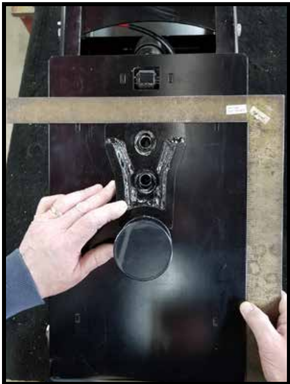
1. Line up the locking plate with the king pin. Square up the back of the locking plate as shown.
