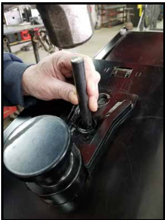
2. Make sure the locking plate does not move. Mark the holes that need to be drilled with a center punch.
