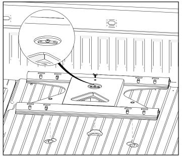
**1.** To install the adapter, remove the bed puck covers if installed. Turn locking turn plate so it is facing side to side as shown.
