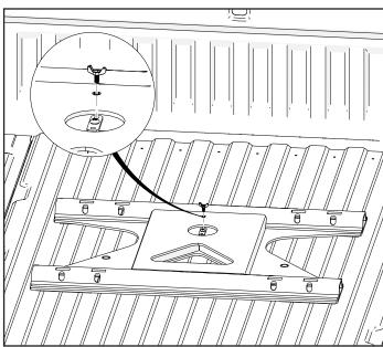
**2.** Lower frame adaptor into the factory pucks. Make sure the frame is fully placed into the pucks. Turn locking turn plate 1/4 turn so it is facing front to back and the locking holes line up.
