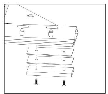
**3.** If locking plate will not turn, that means the hitch can't go down far enough to lock. Remove the two screws from the four pads and remove one or two spacers between the plastic foot pads and reinstall frame until turn plate can turn into the locked position.
