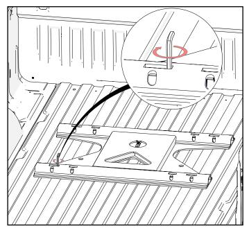
3. Used the hex wrench to adjust the four pads/feet to remove any play/rocking from hitch adapter. Reverse steps to remove.
