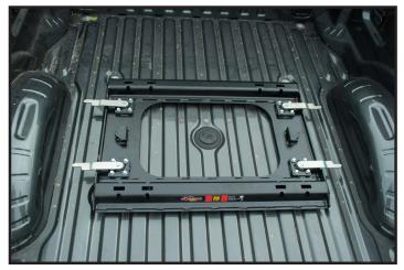
**1.** To fit the frame for the truck pods, remove covers from each mounting pod and with the locking arm bolts loose enough to move the locking mounts, place main frame into box of truck over mounting pods so the locking arms fit into the truck pods as shown. On first install, make sure the four bolts on the the four latches are loose before installing.
