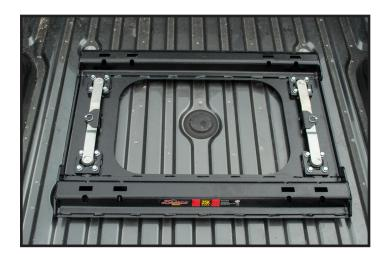
**4.** Place locking pins in mounting holes to lock the latch handles as shown. You are now ready to install your hitch.
