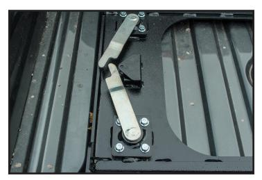
**3.** Once your latches are setup for your truck, turn handle in so they will lock into each other as shown in picture.
