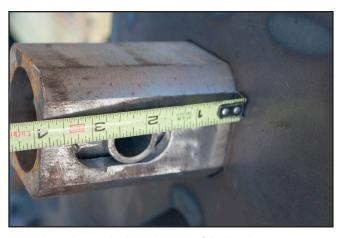
**2.** Adjust the top bolt so the top of the bushing measures approximatly 1/16" less than the measurement from the straight edge to pin. Pull the B&W pin and install adapter into the socket. Allow the B&W hitch pin to slide back into place. If pin in not fully going back into place, the adapter my need to be adjusted.
