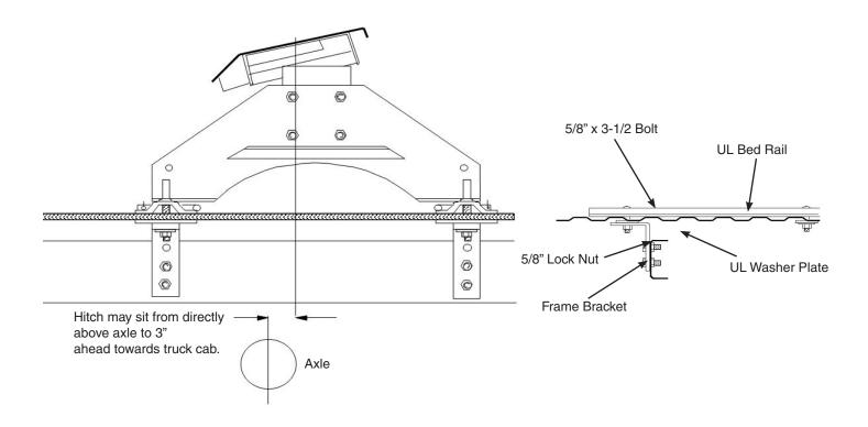
**IMPORTANT NOTICE:** This installation may require different frame brackets for the various truck models. This kit does not contain any frame brackets for this reason. Frame specific installation instructions are available at our website www. towdemco.com or by calling (800)543-3626. Optional brackets are shown below.
