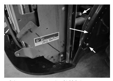
**2.** Loosen or remove engine shield during installation process.
