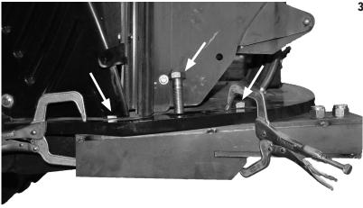
3. Install Right Baseplate using 7/8" x 3.00" Bolts with 7/8" Nylon Lock Nuts. Tighten to 420 ft-lbs. Repeat for the left side.
