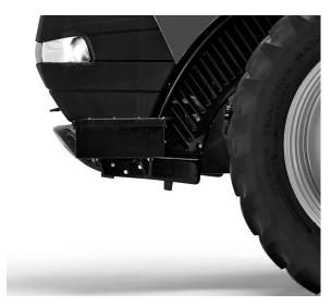
**1.** Remove step/toolboxes brackets and front weight.
