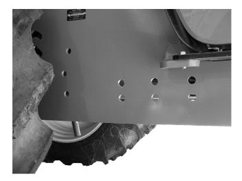
**1.** Install John Deere's front axle support kit for tractor mounted tanks.
