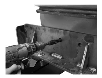
Center punch the drilled hole location and use a 29/32" drill bit to drill holes. Be sure to check for hose clearance on reverse side before drilling.
