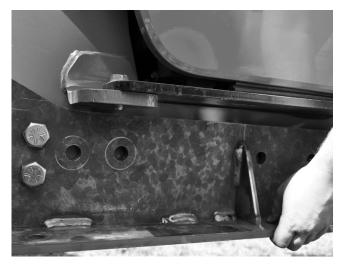
2. Install the right baseplate using 7/8" x 3.00" bolts and nylon lock nuts. Repeat for opposite side. Tighten 7/8" bolts to specified torque found on front cover.
