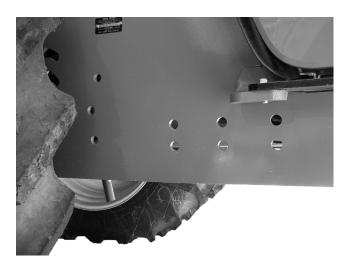
**1.** Install John Deere's front axle support kit for tractor mounted tanks.
