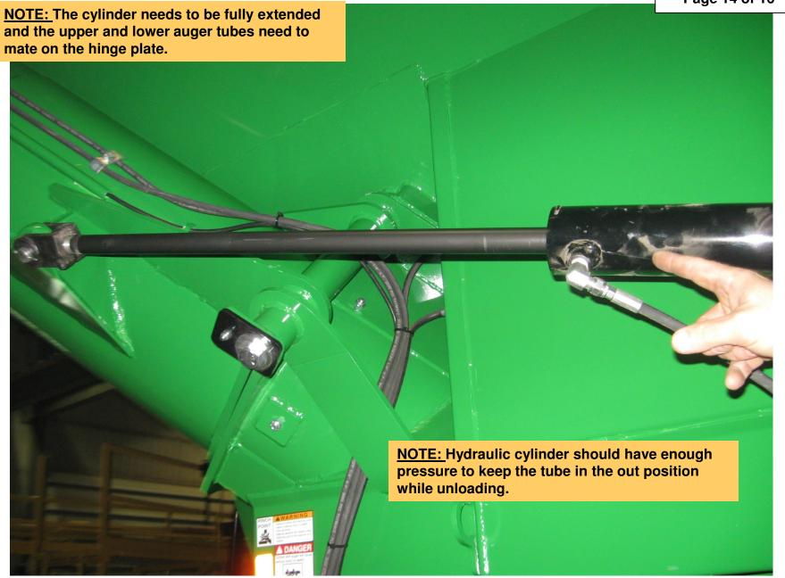
When the cylinder is adjusted properly tighten the jam nuts
