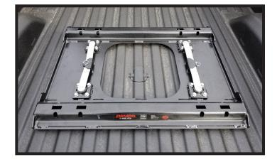
**4.** Place locking pins in mounting holes to lock the latch handles as shown. You are now ready to install your hitch.
