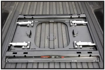
**1.** To fit the frame for the truck pods, remove covers from each mounting pod and with the locking arm bolts loose enough to move the locking mounts, place main frame into box of truck over mounting pods so the locking arms fit into the truck pods as shown. On first install, make sure the four bolts on the four latches are loose before installing.
