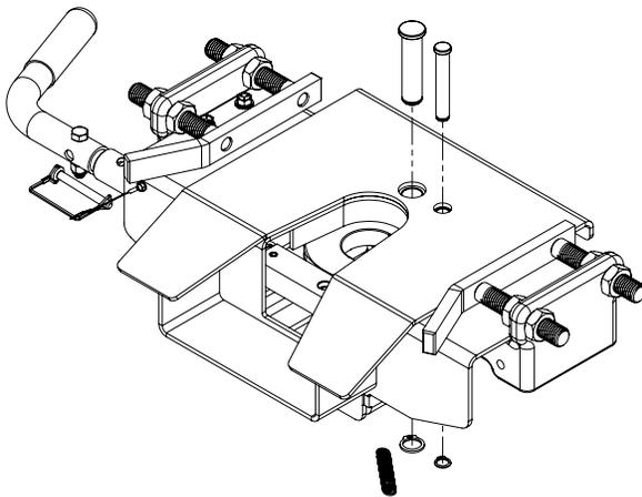
Jaw pins can be removed and greased by removing or unhooking jaw spring and both snap rings. Tap the pin up from bottom. Clean pins and inspect for wear, apply light coat of grease and reinstall pins, snap rings and spring.
