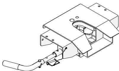
Remove safety lock pin if installed and pull handle until jaw locks open.
