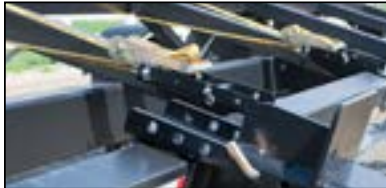
Two fully adjustable ratcheting straps for securing all brands of heads
