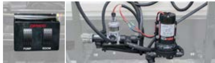
6351 Control console Electric pump and boom control
