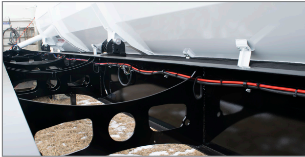
BRAKE LINES Strategically located and color coded
