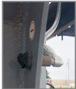
REMOTE GREASE ZERKS Access grease zerks without having to leave the ground
