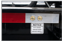
GREASE ZERKS 5th Wheel Plate and a safe and convenient way to grease the Hydraulic Cylinders
