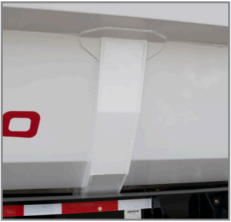
TUB SUPPORTS 3 outer tub supports to increase strength
