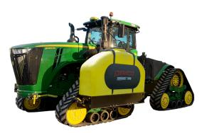
If your tractor is on tracks, we have the perfect product for you: the 1000 Gallon SideQuest<sup>®</sup> Track Unit, which mounts easily on most larger tractors. Featuring two 500 gallon tanks with a 16" fillwell, these Demco saddle tanks are just what you need for your tractor on tracks.
