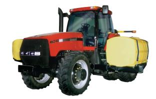
The tanks are made from slim-line polyethylene and feature dual jet agitation, sump, molded sight gauge and fillwell with a no-splash cover, as well as a poly baffle. Farmers love our high clearance brackets. Furthermore, our centrifugal plumbing kits feature single section or three section electric controls.
