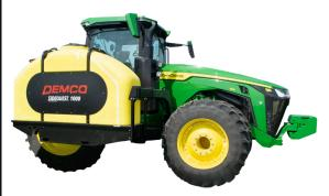
But if you don't need 40" row spacing, check out the Demco 1000 Gallon SideQuest<sup>®</sup> Side Mount saddle tanks. These SideQuest<sup>®</sup> tanks come with a 16" fillwell and mount on an extended rear axle spindle to better distribute weight (75 percent to rear, 25 percent to front), which **relieves stress on your tractor's axles** (dual rears required).
