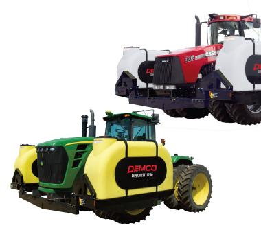
Doubles the capacity of our Quick Tach to 1,200 gallons. This high capacity system comes with a 16" fillwell and better visibility due to their longitudinal design.
