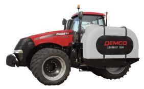
When 40" row spacing is needed, consider the Demco 1000 Gallon SideQuest<sup>®</sup> - 40" Row Spacing tractor mounted fertilizer tanks. With a 16" fillwell and an extended rear axle spindle mount that moves more weight to the rear (rear duals required), your tractor should enjoy a long life of operation with Demco tractor mounted tanks.
