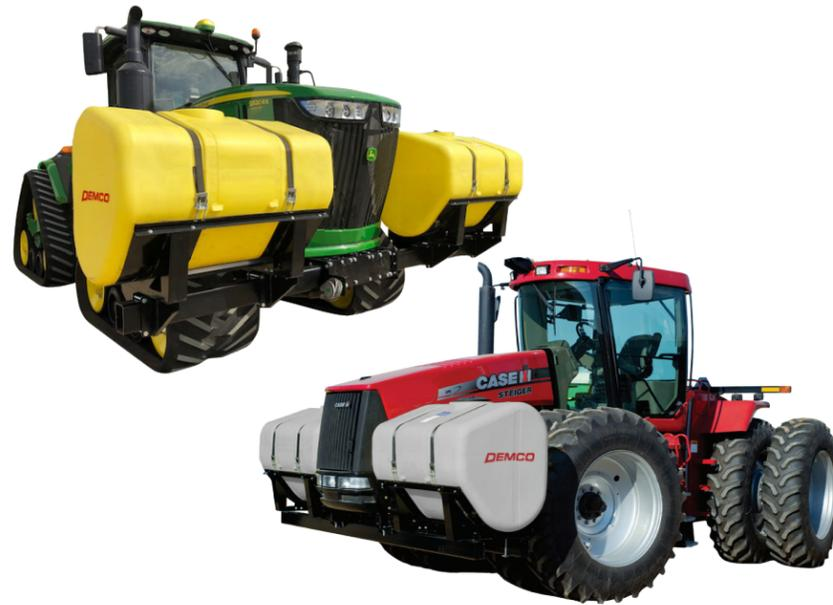
By retaining driver visibility and featuring about two feet of ground clearance, Demco tanks are as usable as they are durable. The tanks come with dual jet agitation, sump, molded sight gauge and a 12" fillwell with no-splash cover.
