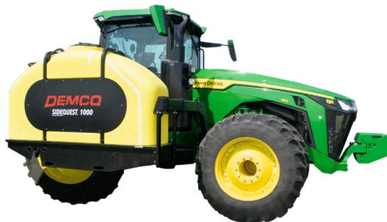
But if you don't need 40" row spacing, check out the Demco 1000 Gallon SideQuest® Side Mount saddle tanks. These SideQuest® tanks come with a 16" fillwell and mount on an extended rear axle spindle to better distribute weight (75 percent to rear, 25 percent to front), which **relieves stress on your tractor's axles** (dual rears required).
