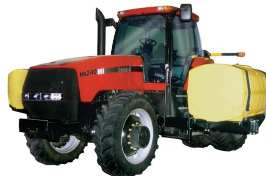
The tanks are made from slim-line polyethylene and feature dual jet agitation, sump, molded sight gauge and fillwell with a no-splash cover, as well as a poly baffle. Farmers love our high clearance brackets. Furthermore, our centrifugal plumbing kits feature single section or three section electric controls.
