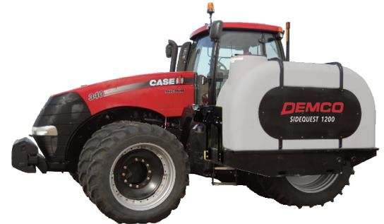
When 40" row spacing is needed, consider the Demco 1000 Gallon SideQuest® - 40" Row Spacing tractor mounted fertilizer tanks. With a 16" fillwell and an extended rear axle spindle mount that moves more weight to the rear (rear duals required), your tractor should enjoy a long life of operation with Demco tractor mounted tanks.
