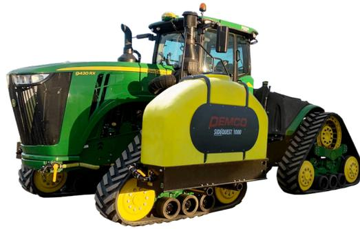
If your tractor is on tracks, we have the perfect product for you: the 1000 Gallon SideQuest® Track Unit, which mounts easily on most larger tractors. Featuring two 500 gallon tanks with a 16" fillwell, these Demco saddle tanks are just what you need for your tractor on tracks.
