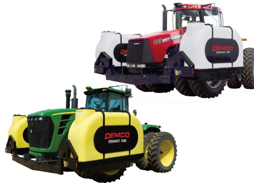
Doubles the capacity of our Quick Tach to 1,200 gallons. This high capacity system comes with a 16" fillwell and better visibility due to their longitudinal design.
