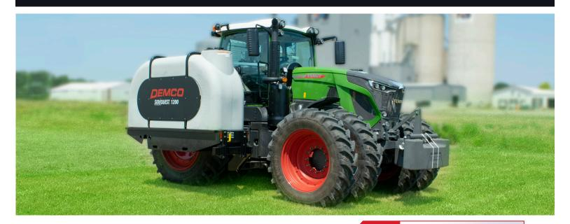
This innovative design features a hub spacer and bearing system for mounting the tank to the outer rear dual allowing weight to be shifted to the rear for less stress on the tractor frame.
