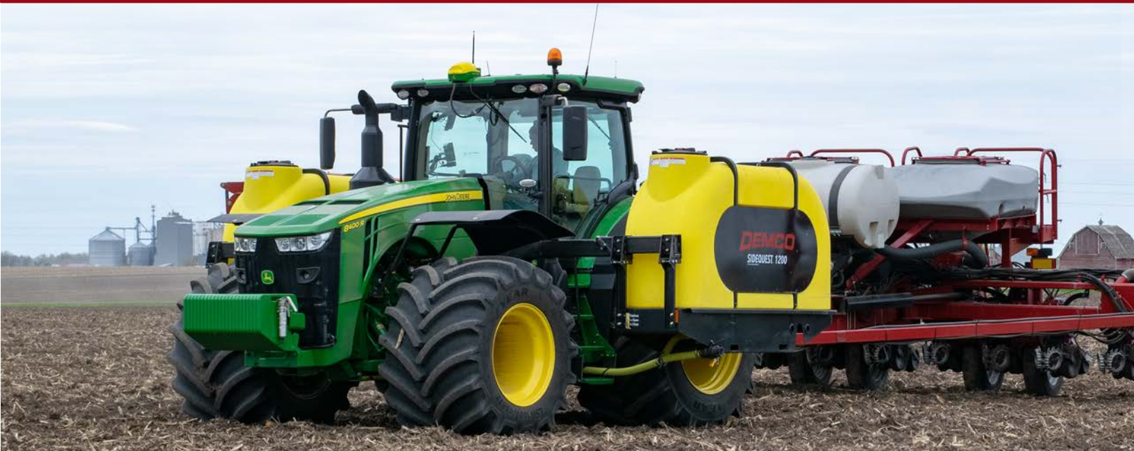
Demco's 300 Gallon Single Axle Sprayer with a 21', 30', or 40' boom has polyethylene elliptical tank with two dual jet agitators and sump.
