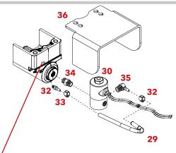
Drill the hole using a 5/32" bit. Hole location is .900" right of top left corner and .900" down from top of master cylinder. Tap hole with 10-32 NF tap
