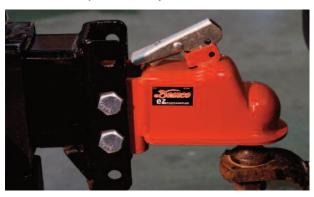
(2) At the mid-way point when lowering the trailer, the stem on the handle will begin to rise up allowing the ball to enter the ball socket.
