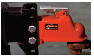
(3) Once the ball has fully engaged the socket the ball keeper will snap back into place securing the coupler to the ball.
