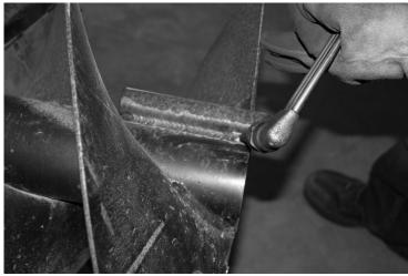
4. Remove Drive Pin from outside of core tube. (be careful not to cut into core tube)
