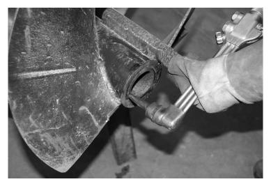
2. Cut weld between inner bushing and core tube (be careful not to cut into core tube).
