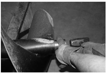
3. Drive bushing into core tube a minimum of 4". Clean up inside diameter of core tube.
