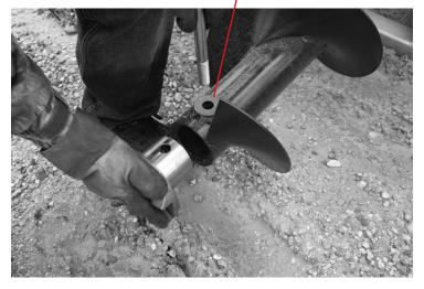
7. Insert outer drive casting (12028 for 800-950, 12188 for 550/650/750) into outer flighting and attach using 3/4" x 6" Hex Head Bolt Gr. 8 (10525) and 3/4" Nylon Locknut (02961). Reinstall outer flighting in outer tube.
