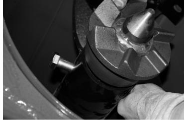
8. Remove old Drive from inner flighting. Remove inner flighting from cart. If inner flighting core tube has 5/8" holes, you will need to drill them out to 25/32". Slide lower Posi-drive into Hanger bearing. Then insert lower Posi-drive into inner flighting and attach using 3/4" x 5" Hex Head Bolt Gr 8 (11099) and 3/4" Nylon locknut (02961). Reinstall inner flighting into cart.
