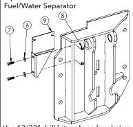
Use 13/32" drill bit and use bracket as drill template. Drill two holes and secure using provided fasterners. Attach filter with existing hardware.
