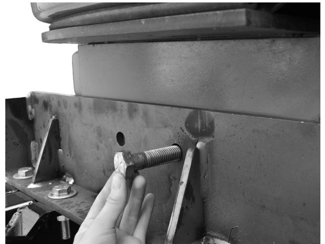
4. Install 7/8" x 3.00" bolts and nylon lock nuts into drilled holes and tighten to specified torque.
