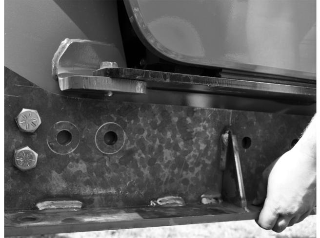
2. Install the right baseplate using 7/8" x 3.00" bolts and nylon lock nuts. Repeat for opposite side. Tighten 7/8" bolts to specified torque found on front cover.
