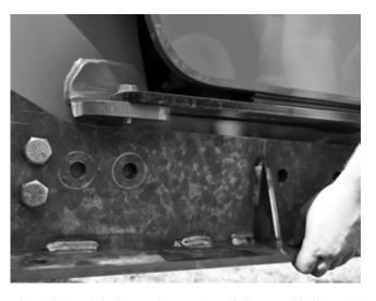
2. Install the right baseplate using 7/8" x 3.00" bolts and nylon lock nuts. Repeat for opposite side. Tighten 7/8" bolts to specified torque found on front cover.
