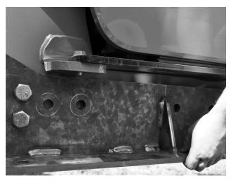
Install the right baseplate using 7/8" x 3.00" bolts and nylon lock nuts. Repeat for opposite side. Tighten 7/8" bolts to specified torque found on front cover.
