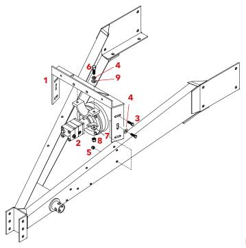
**40.** Begin by bolting the pump hanger (#1) to the frame with four 3/8" x 1-1/4" bolts, two flatwashers and four nylon locknuts as shown.
